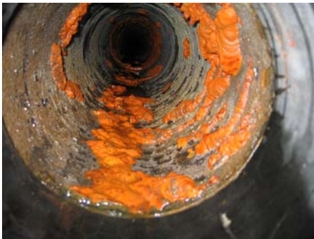
Fig-4a) and 4b) Showing internal scale in cast iron water pipe
