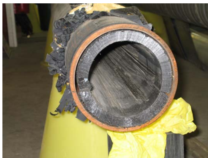
Fig-7a) 19mm HDPE liner in 200mm steel pipe
