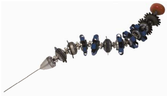
Fig-6a) (above) showing a tethered RFT tool Fig-6b) (right) showing a free-swimming RFT tool
