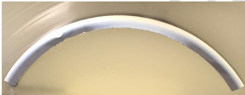
Fig-3: 5-Chrome tube with external carburization (light area)
