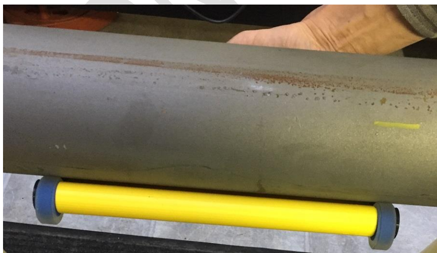
Fig-1: CIRC E-PIT probe on furnace tube
