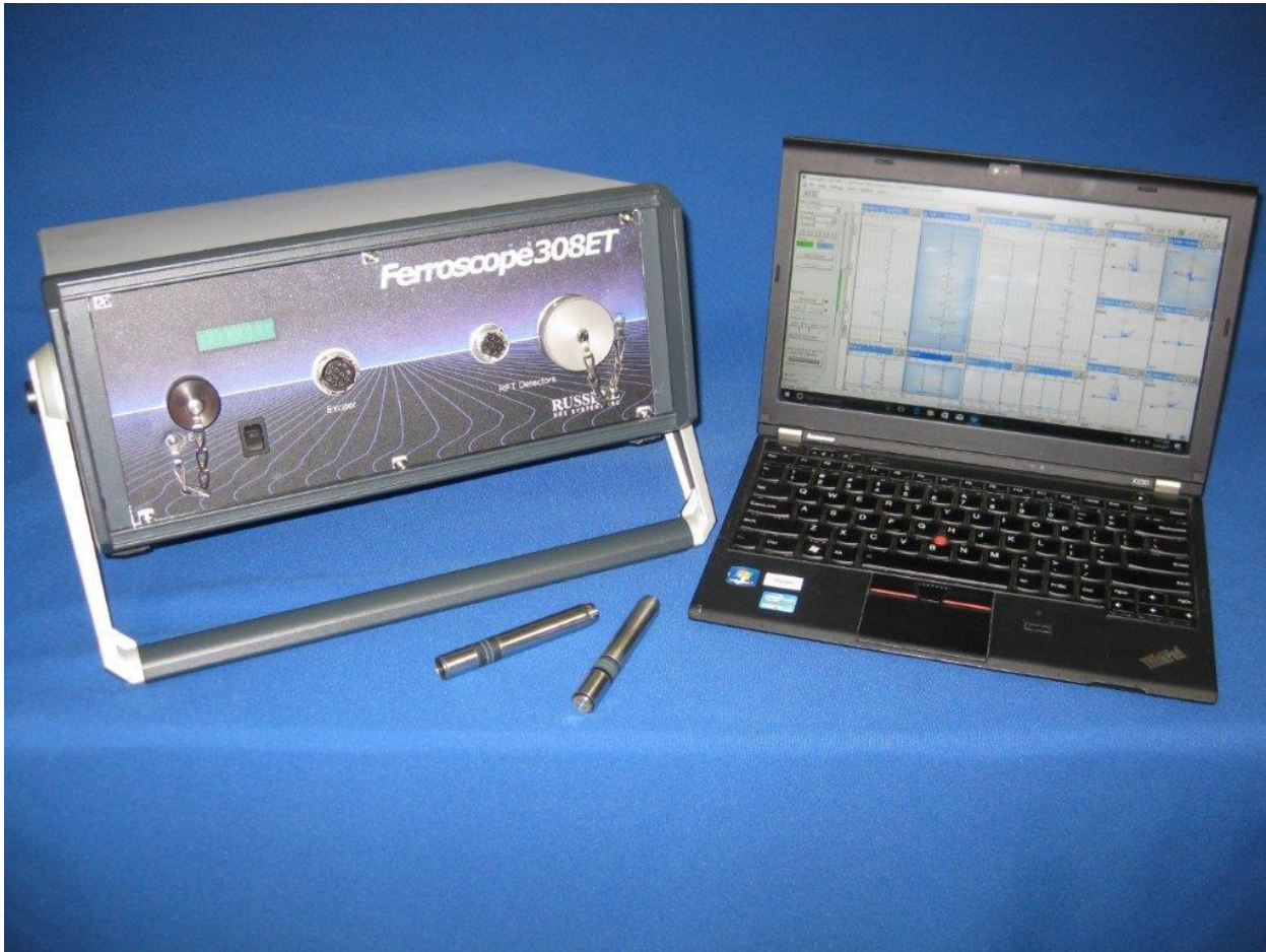
Fig-4: Ferroscope and lap-top computer used with CIRC E-PIT probe
